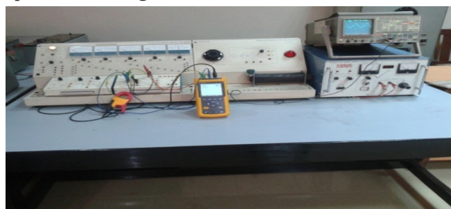
Fig. 5. Experimental setup of AC voltage converter
